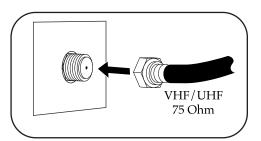
Connect the 75 ohm cable from the combination VHF/UHF antenna to the antenna jack.
