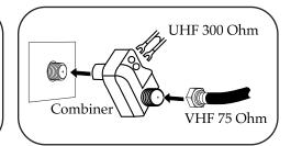
Connect the 75 ohm cable from the VHF antenna and the UHF antenna twin-lead wire to a combiner (NOT SUPPLIED). Attach the combiner to the antenna jack. **NOTE:** If your VHF antenna has a twin-lead wire use a 300-75 ohm matching transformer, then
